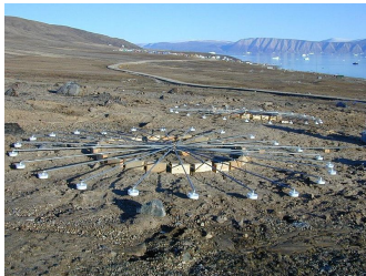
CTBTO Infrasound Array, Greenland
